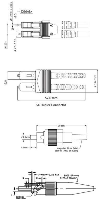
**B&C Fiber Group** duplex patch leads are manufactured in our own modern facilities from the highest quality optical fiber, terminated with ceramic ferrule connectors of various types. Cable preparation, termination and performance testing is carried out to strictly managed procedures, with high focus on quality control.
