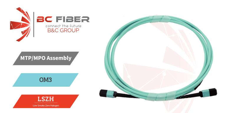
MTP and MPO patchcords are constructed from a 12-fiber round mini-core cable, which has a minimal cable diameter while offering excellent bending flexibility. It is preterminated with a 12-fiber MTP connector on both ends, with customer-specified cable type and length. This high density patchcord type can be used to speed up installation, minimize errors and reduce space.
