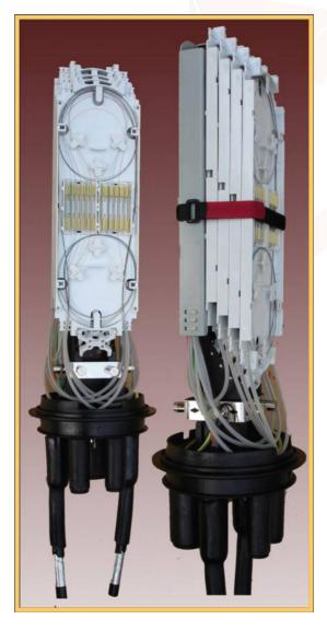
M2 is designed for both single fiber and ribbon fiber. Excessive fibers can be stored in storage basket behind the splice trays. Per closure can accommodate up to 4 pieces of trays.
